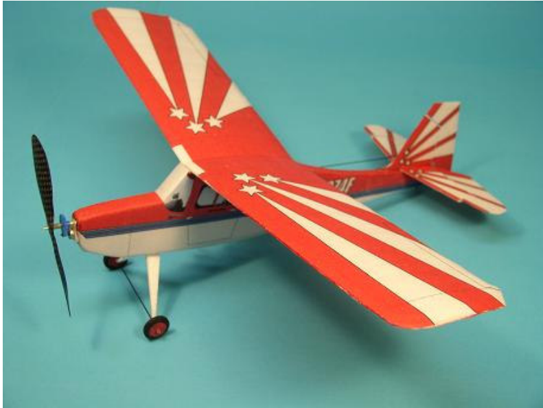
The PU03 propulsion set is put to good use in my 13-inch span, 16.8g, all Depron semi-profile Citabria.
