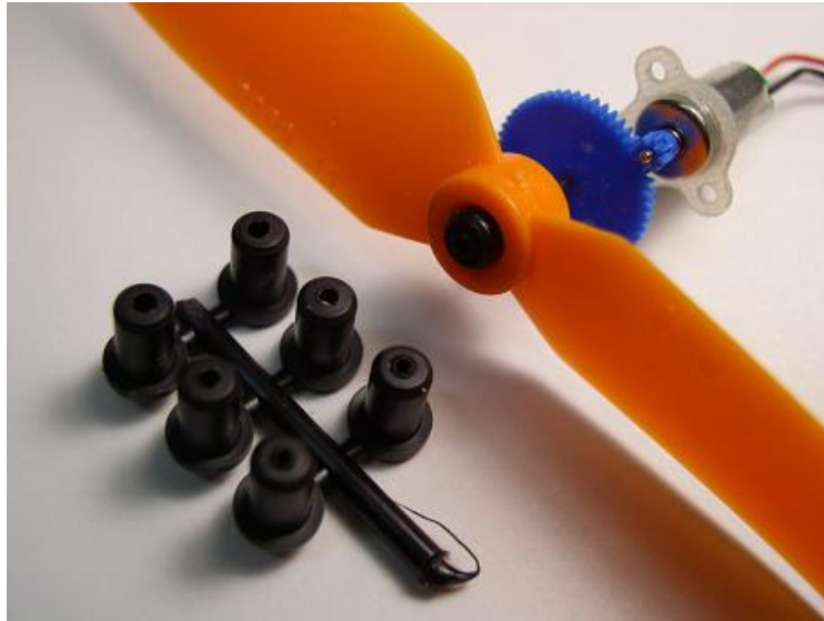
The new Bob Selman Designs prop adapters. Two of the six adapters allow the popular GWS 4mm bore props to be used with a 1mm shaft.
