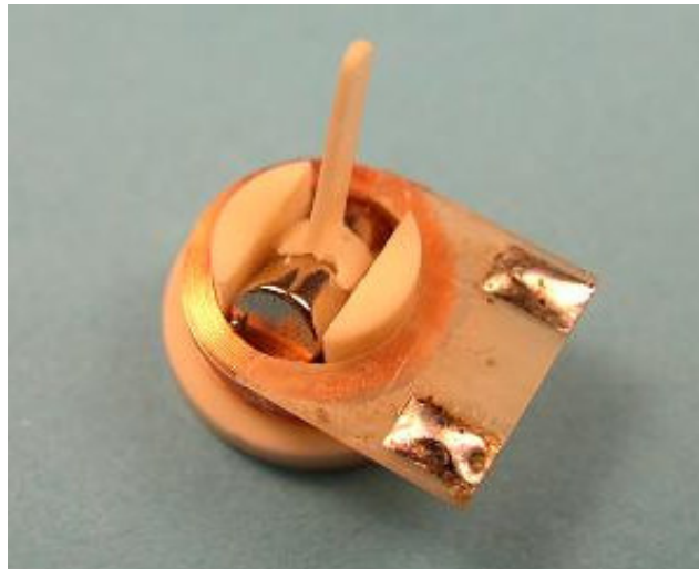
The JMP Actuator (shown with a prototype housing) weighs 1.4g and generates 2.9 g-cm torque at 3.5 volts.
