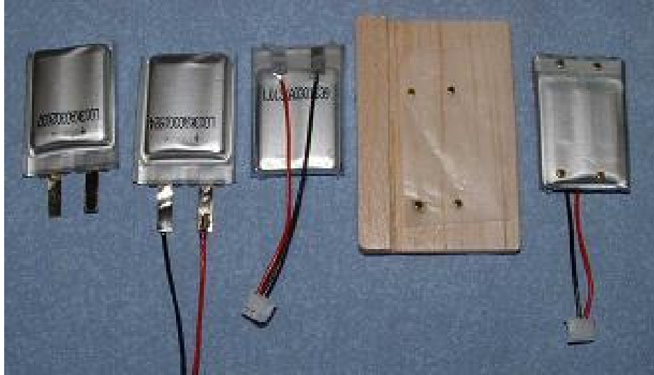
From left to right, the steps I follow to make a single-cell LiPoly battery pack. (1) solder the leads onto terminals that have been brushed with electronics soldering flux; (2) tape the terminals with cellophane tape and fold back over top of cell and encase in clear shrink; (3) place magnets on template covered with wax paper and then glue to shrink wrap covering the cell.
