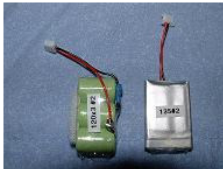
Shown on the left is the old standard, a 3-cell 120mAh NiMH battery pack which weighs 11.8g. On the Right is a new 135mAh LiP battery, which weighs 4.1g. I label each of my battery packs and keep a log to monitor each pack's charging history.
